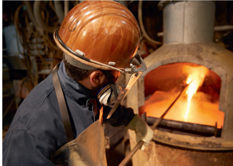
▲ Slag is tapped from the furnace and very largely returned to the process, after cooling
