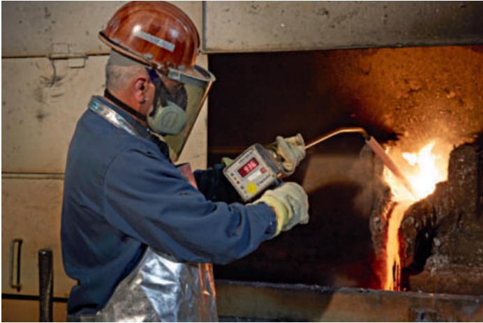
▲ Raw lead is melted out of the used batteries and is cast after intermediate cooling into ingots in moulds. Checking of temperature is one of a number of regular quality controls performed during this recycling process
