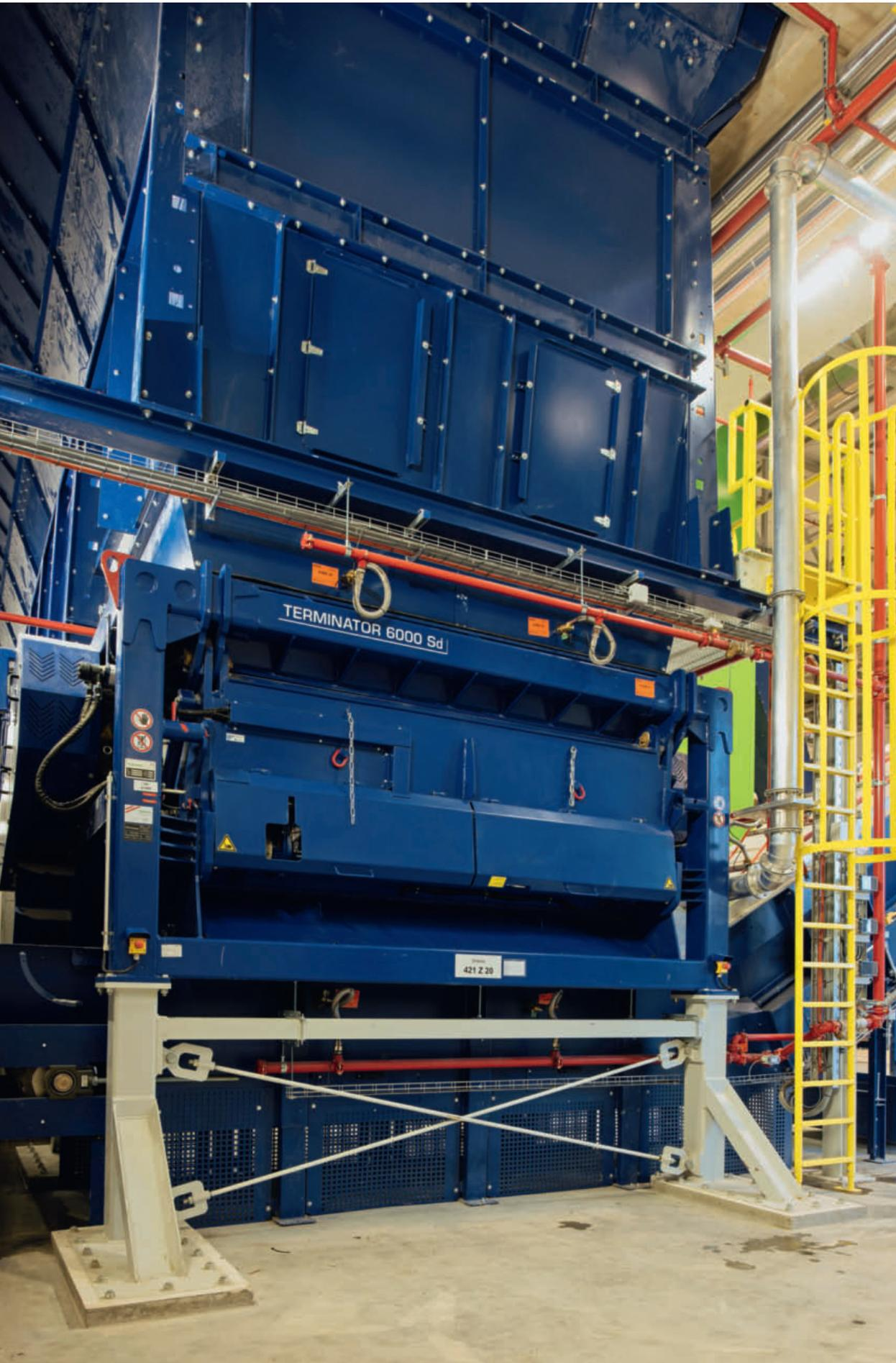
◀ The Terminator is a key component – as pre-shredder, it must deliver a consistent particle size for all downstream processing steps
