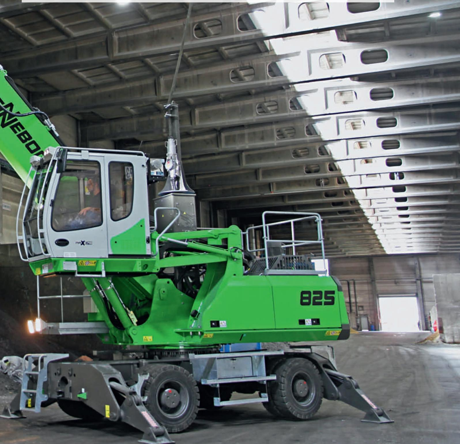
Whether in material sorting or in loading trucks. Thanks to ceiling current supply, the SENNEBOGEN 825 electric material handler can be flexibly used indoors
