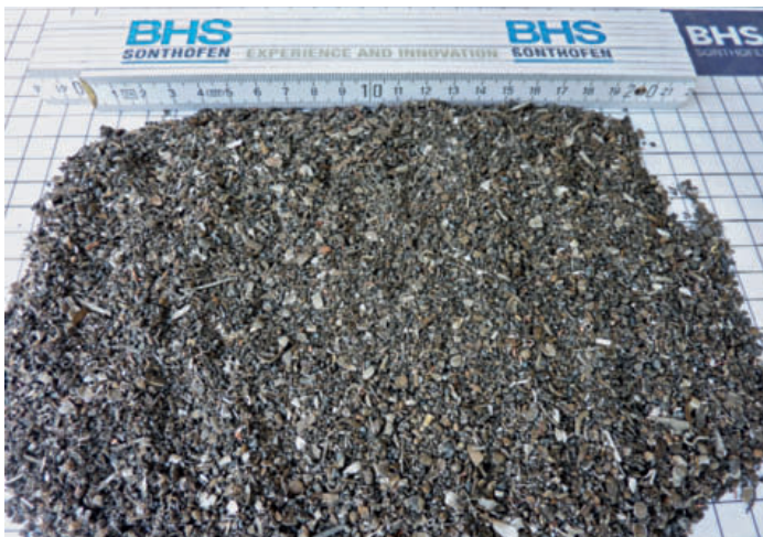
▲ 8a Output material (example): magnetic metal fractions with a particle size between 0 and 3 mm
