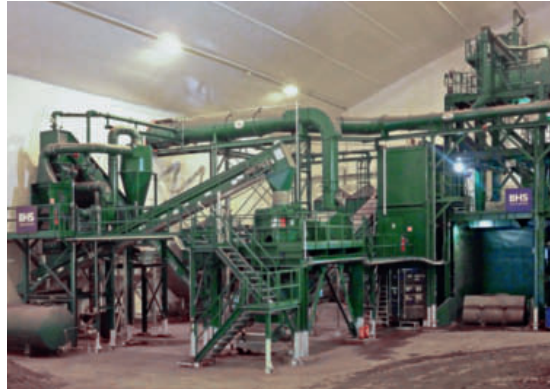
2 The centerpiece of the new ASR recycling plant: the BHS rotor impact mill (RPMV)
