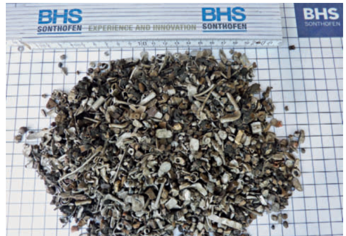
▲ 8b Output material (example): magnetic metal fractions with a particle size between 3 and 6 mm
