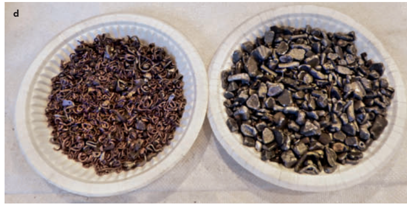
◀ 9c Output material (example): non-ferrous metal with a particle size between 3 and 6 mm, separated into heavy fraction (left) and light fraction (right)
