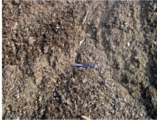
◀ 7 ASR input material with a particle size between 0 and 30 mm used in processing fine fractions
