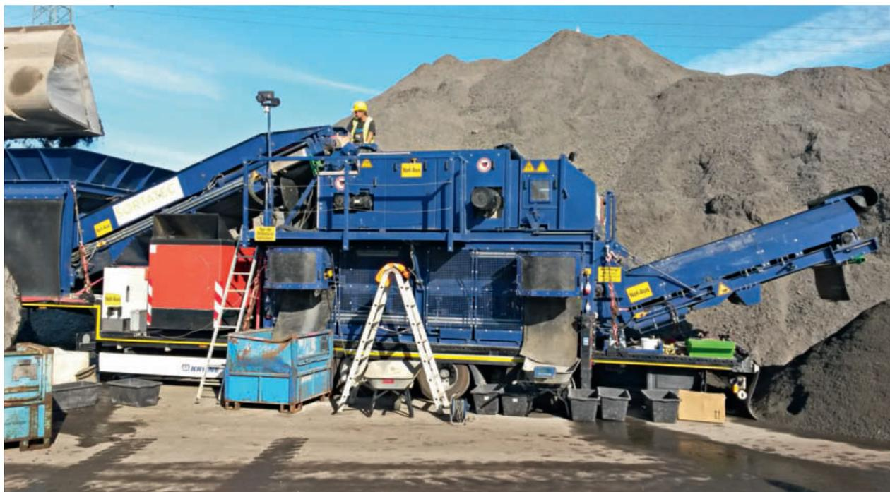
magnetic field penetration depth all boost the separation efficiency for both the fine (< 5 mm) and medium metal fractions – in many cases by up to 30 %.
