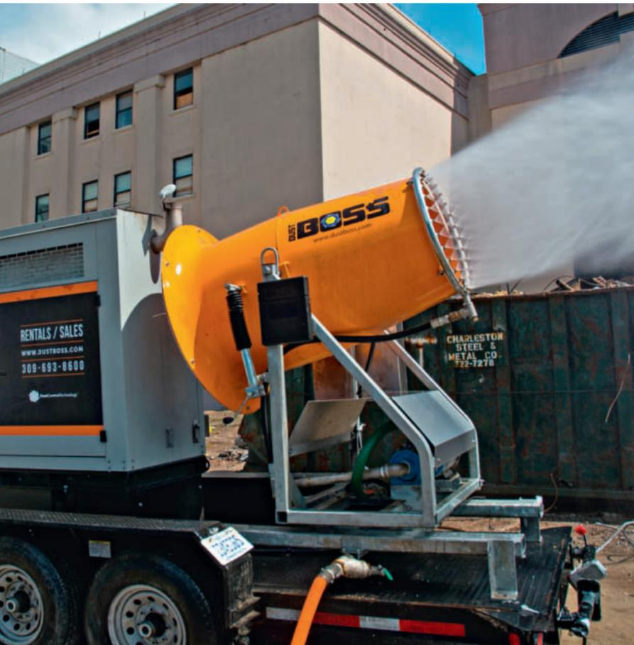
*Atomized mist effectively suppresses fugitive dust in the air and on the ground, without excessive runoff*
