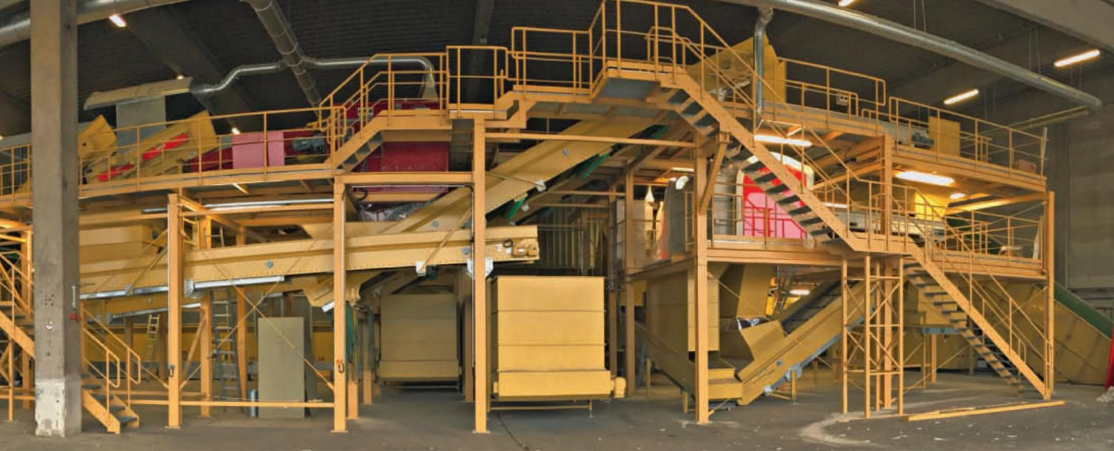
input material (i.e. the amount of cardboard). The downstream sorting units can therefore operate at any time with the highest efficiency. After the storage bunker the input material flow is split up evenly into two lines in order to achieve an optimum distribution of the material.
