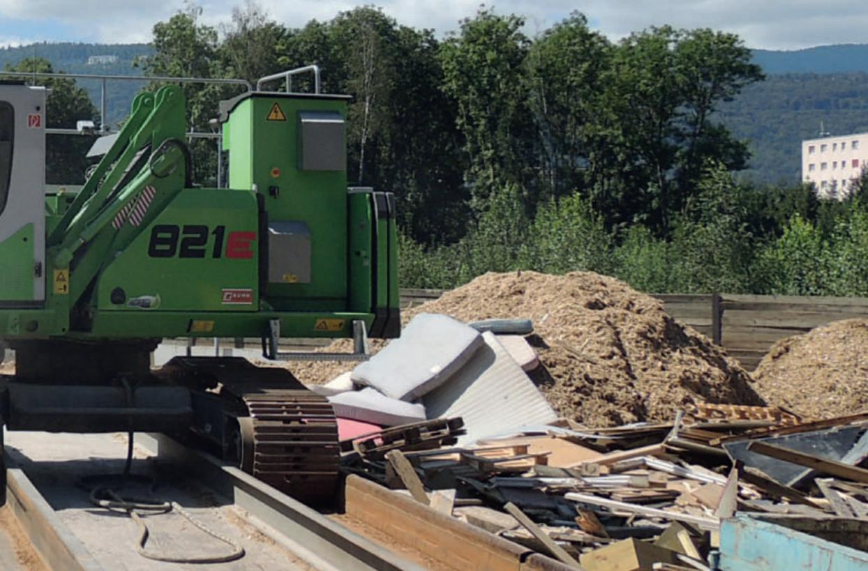
◀ A SENNEBOGEN 821 with crawler traveling gear at Remo AG
