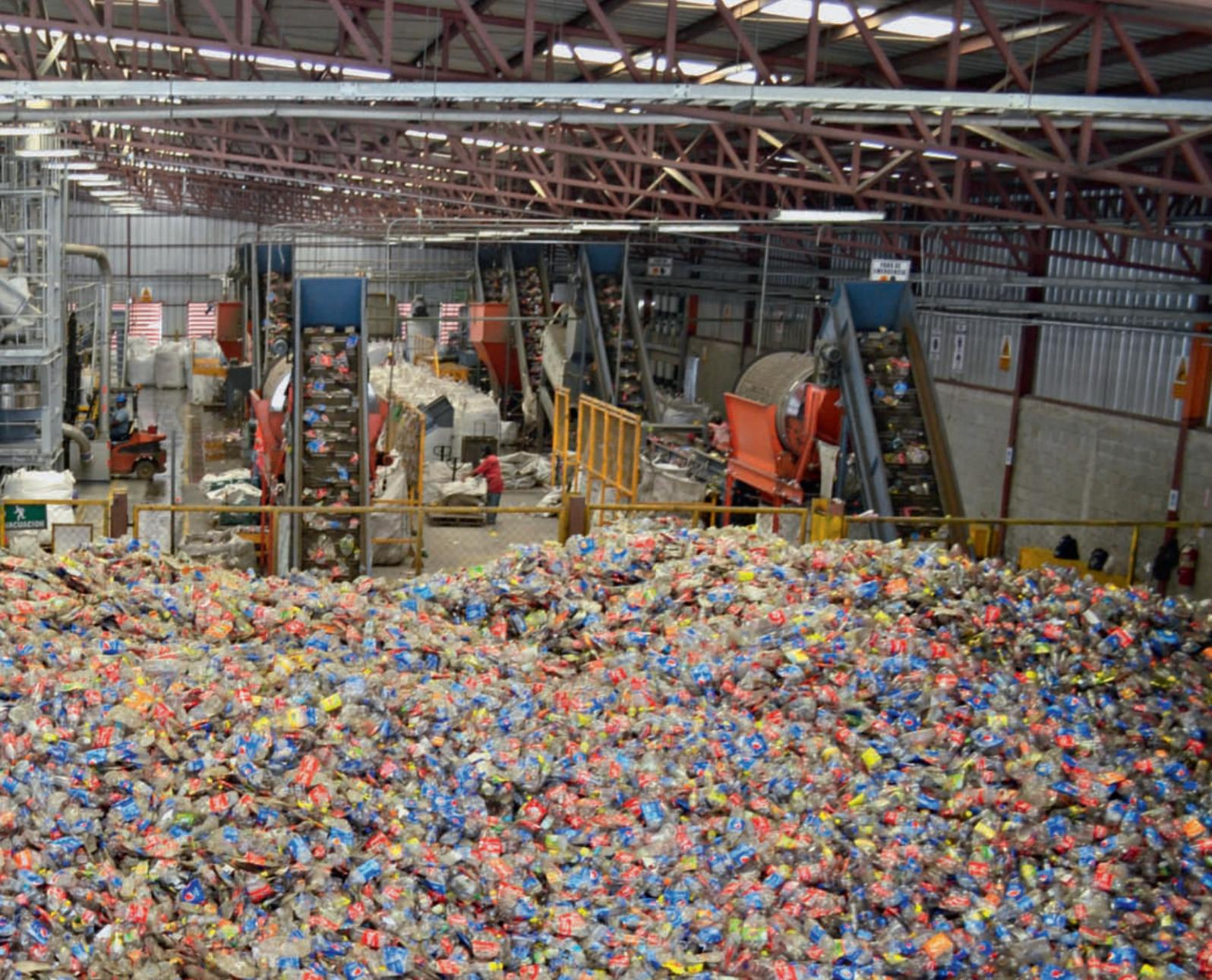
In a multi-stage process, the bottles are pre-sorted, size-reduced, washed cold and hot and after drying forwarded to a flake sorting step. The German machine manufacturer Herbold Meckesheim produced, installed and commissioned the plant.
