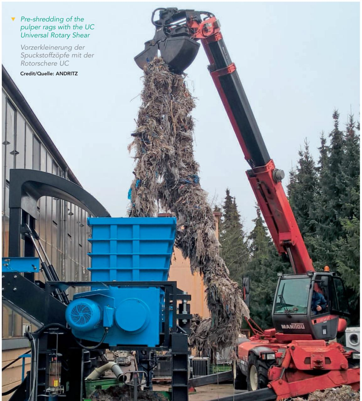
ANDRITZ MeWa will supply a two-stage process for treatment of the pulper rags. In the first section of the plant, the rags will be pre-shredded using the Universal Rotary Shear UC 1300. The slowly rotating, twin-shaft cutter unit is excellently suited for powerful and, at the same time, energy-saving pre-shredding of the stringy input material and is largely insensitive to potential impurities.
