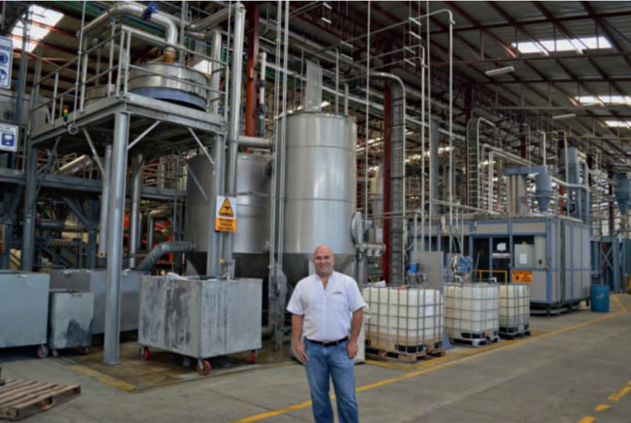
▲ After sorting, the PET bottles are size reduced in two Herbold granulators with a capacity of 1800 kg/h each
