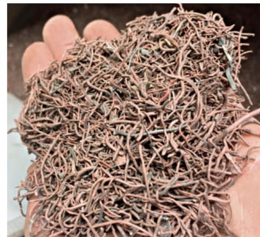
The three individual sizes are then fed to the three-way separating tables. In each individual three-way separating table, either the remaining organic constituents are removed again or the heavy metals are separated off. The metal fractions larger than 4 mm can optionally be prepared in an optical sorter. The aluminum parts and copper cables are then separated using a color-based sorting process.
