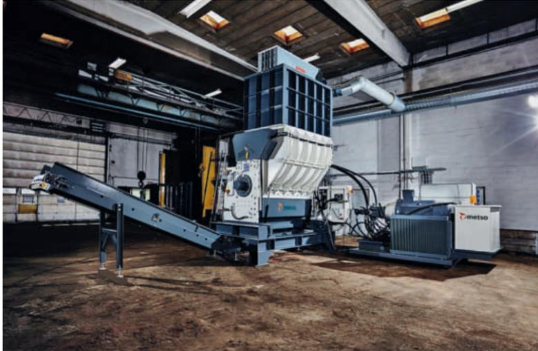
For ideal RDF production, Metso's new fine-shredders are equipped with a single shredding shaft with vertical feed by a pusher. The patented knife system and carefully engineered pusher generate less heat, and minimal downtime in production is secured with durable parts and easy access for maintenance.
