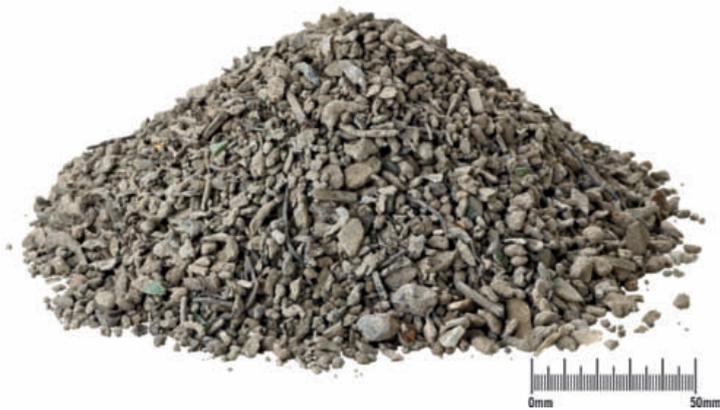
▲ DHZ feed material: non-ferrous metal fractions sized 0–3 mm
