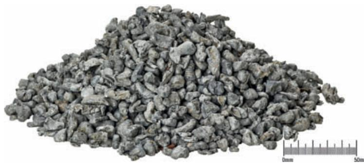
▲ DHZ output: light fraction with dimensions from 4–10 mm delivered by the second 'fine processing' line
