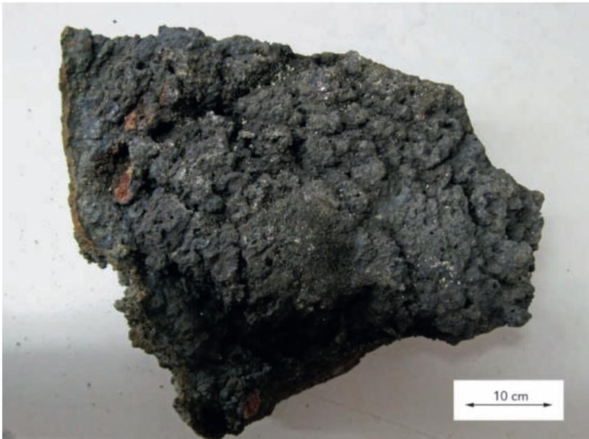
Slag material with very high grinding hardness
