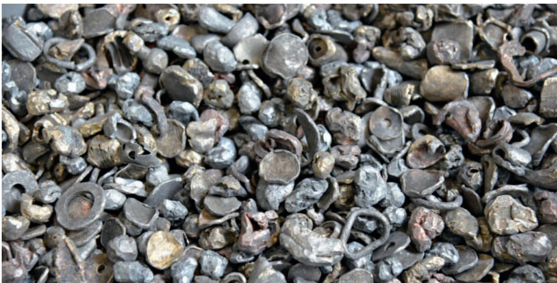
◀ *The high-purity heavy-metals fraction consists mainly of a mixture of copper, brass and zinc*
