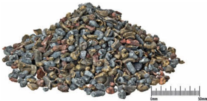
▲ DHZ output: heavy fraction with dimensions from 4–10 mm delivered by the first processing line
