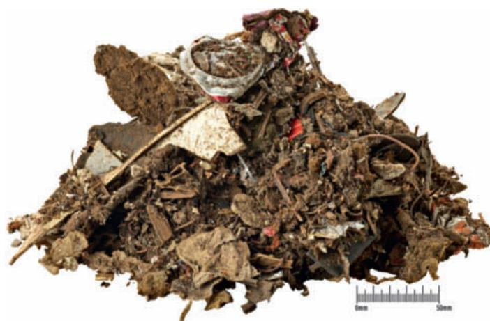
▲ DHZ feed material: shredder residue
