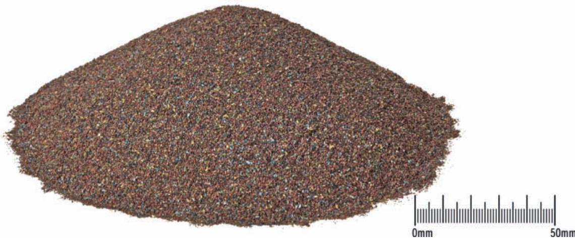
DHZ output: light fraction with dimensions from 0.3–0.8 mm delivered by the second 'fine processing' line
