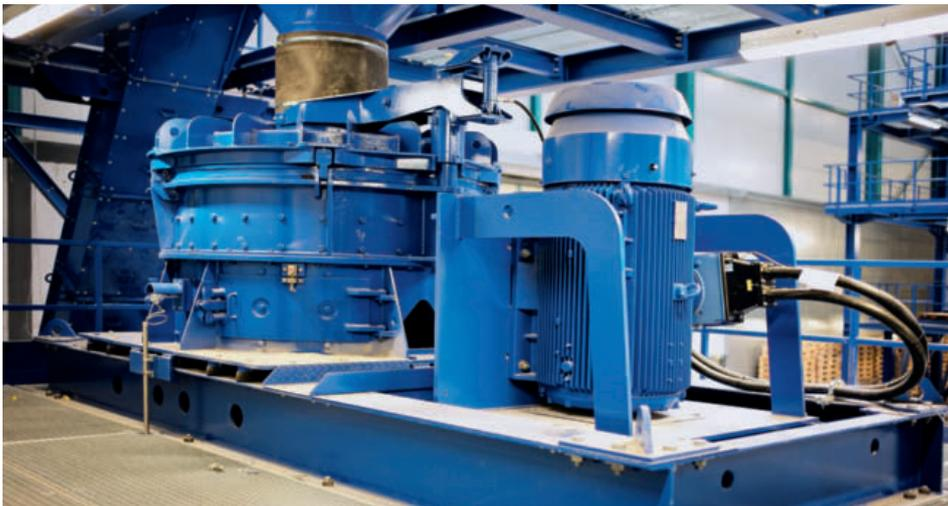
▲ For the fine processing of non-ferrous metals in incinerator bottom ash the two BHS rotor impact mills of type RPMV 1113 and RPMX 1516 are central components of the plant
