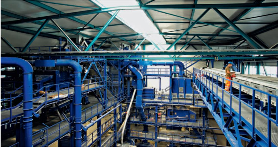
◀ The BHS delivery scope comprised all components for two entire processing lines: from feeding systems and machine technology through to the big bag loading station
