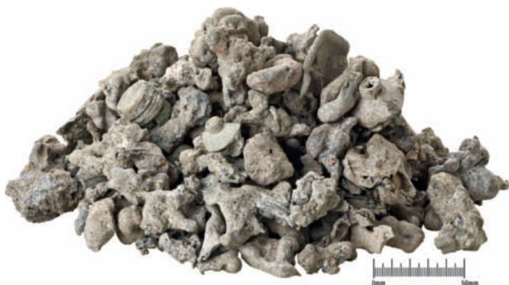
▲ DHZ feed material: non-ferrous metal fractions sized 12–40 mm
