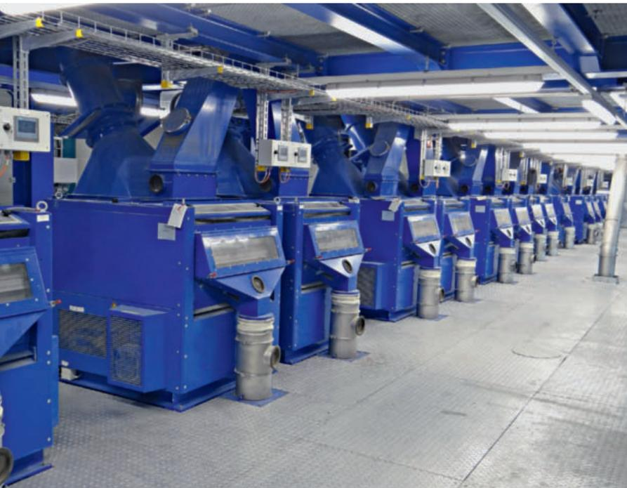
*Density-based separation is used to separate the non-ferrous metals mixture into a lightweight and a heavy-metals product. A total of fourteen modern density-based sorting machines are used for this purpose*
