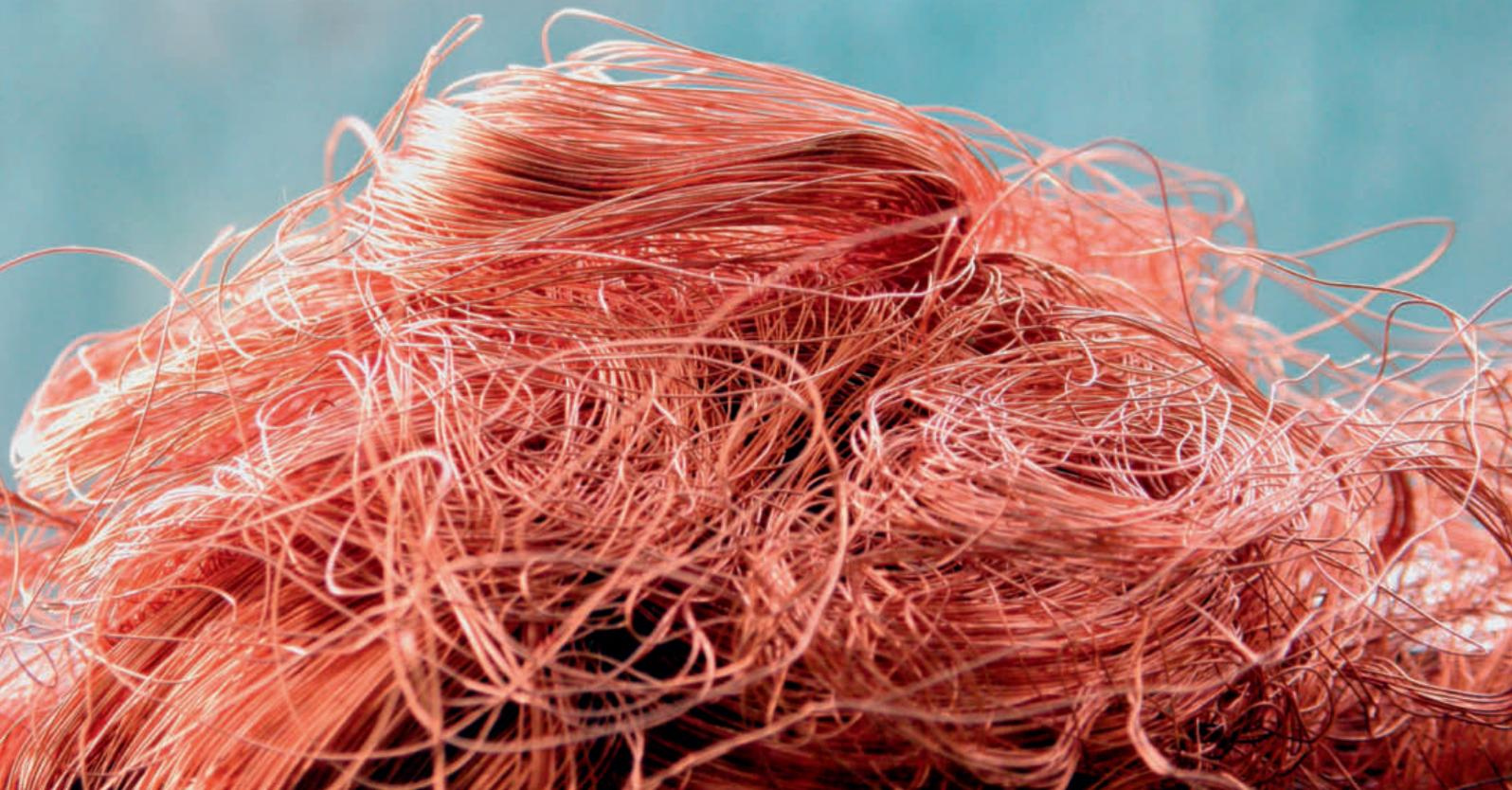
**Bare copper wire** ▲ FRHC copper rod production process can tolerate scrap feedstock with higher impurities which are removed via thermal refining.
