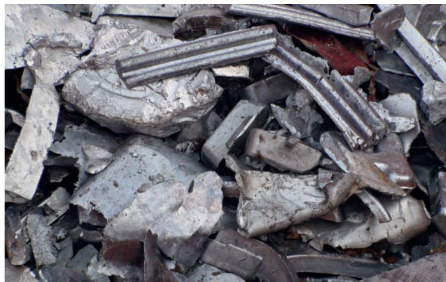
material is free-flowing after comminution and has a multiple of the original bulk weight.
