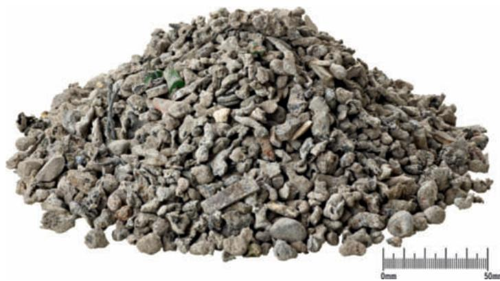
▲ DHZ feed material: non-ferrous metal fractions sized 3–12 mm
