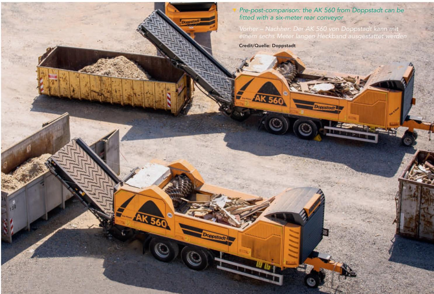
▼ *Pre-post-comparison: the AK 560 from Doppstadt can be fitted with a six-meter rear conveyor*
