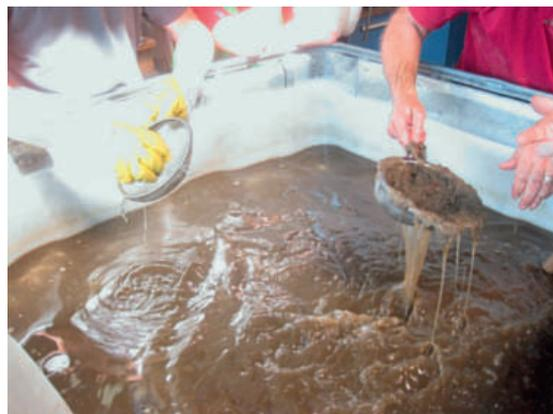
◀ The sink/swim process separates, for example, heavy sand grains from lighter plastic particles
