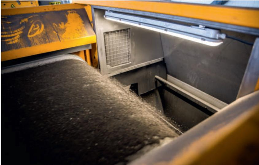
4 ▲ *The flip-flow feeder feeds the material to the NF sorting plant*
