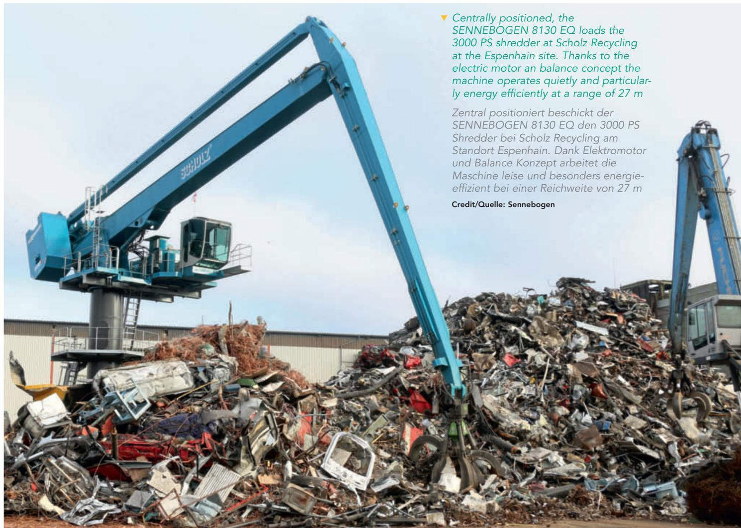
▼ Centrally positioned, the SENNEBOGEN 8130 EQ loads the 3000 PS shredder at Scholz Recycling at the Espenhain site. Thanks to the electric motor an balance concept the machine operates quietly and particularly energy efficiently at a range of 27 m
