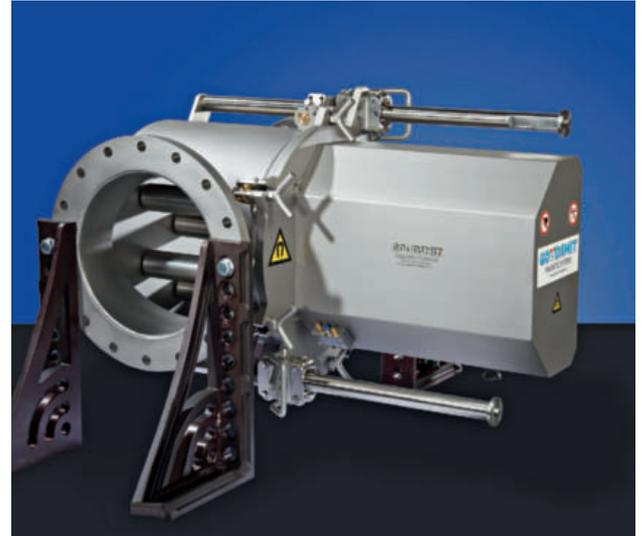
Magnetic filters remove baling wire from paper pulp and prevent damage to equipment and production downtime
