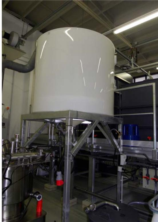
◀ 10 Reactor for wet-chemical digestion
