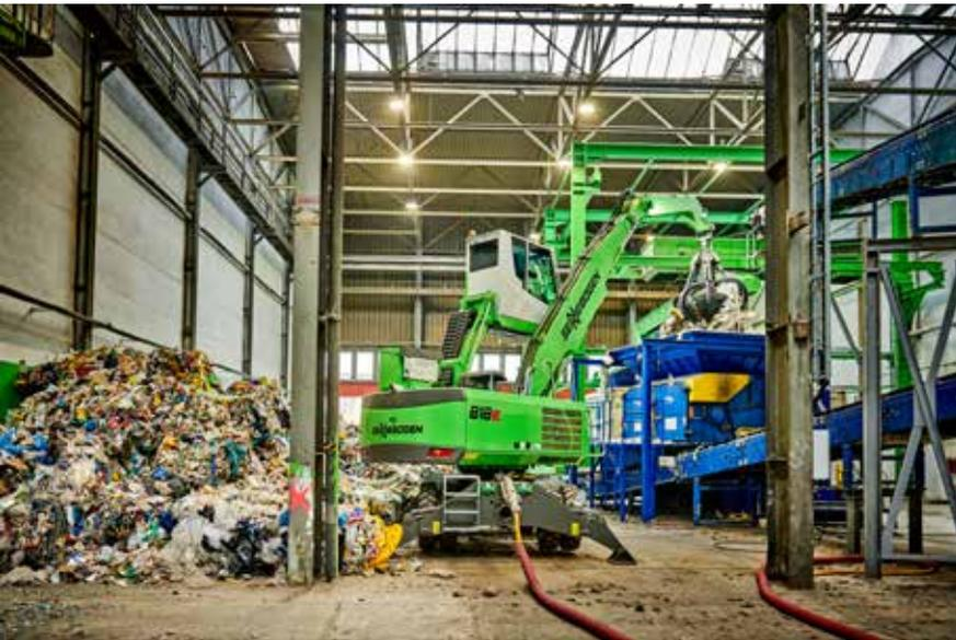
◀ Rear view of the 818 M Special – strain-relieved cable with power supply from the side walls of the hall
