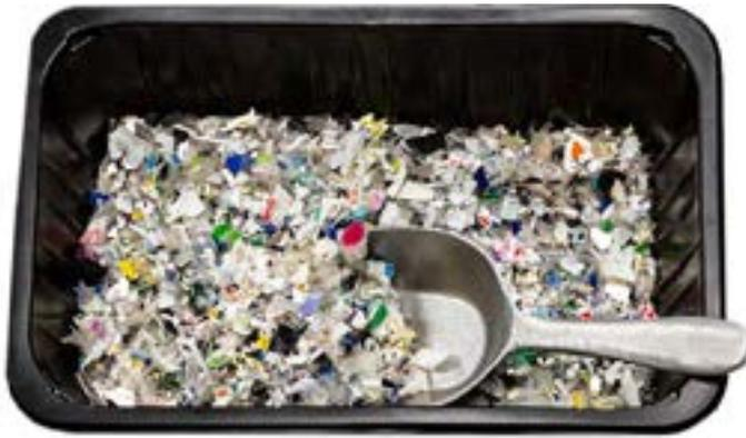
◀ The regranulates come from plastic waste from the dual systems in Germany
