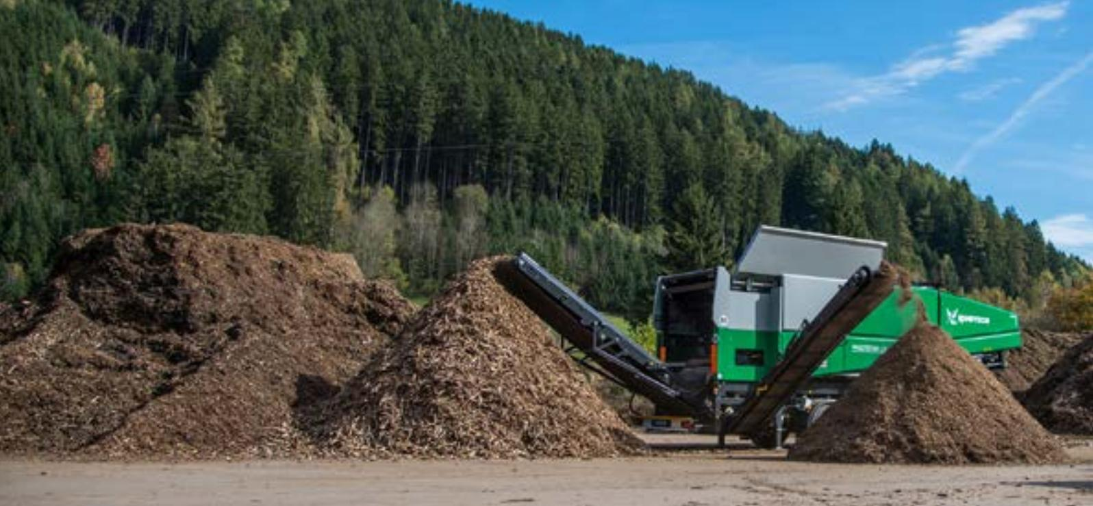
*High flexibility, simple maintenance, toughness, intuitive operation, and design to match are the major features that determine the functionality of the Multistar L3*
