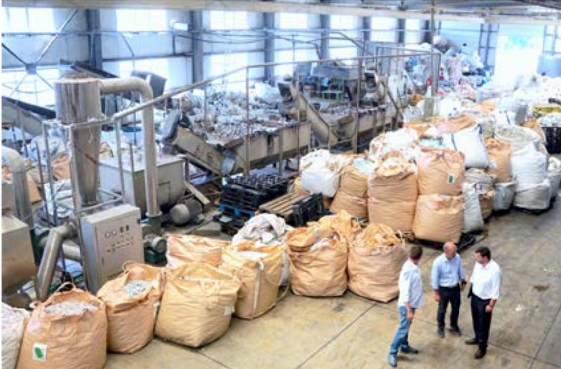
◀ A meticulous material processing with shredding, washing and drying is the basis for the Kaskada quality granulates. To this end, several preparation lines are in operation
