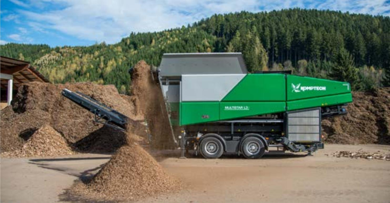
design of the screen decks means they can be removed as a unit and switched in a very short time. This simple removal makes maintenance, conversion and particle size changes easier, and represents a major increase in the machine's flexibility, especially in terms of grain size.
