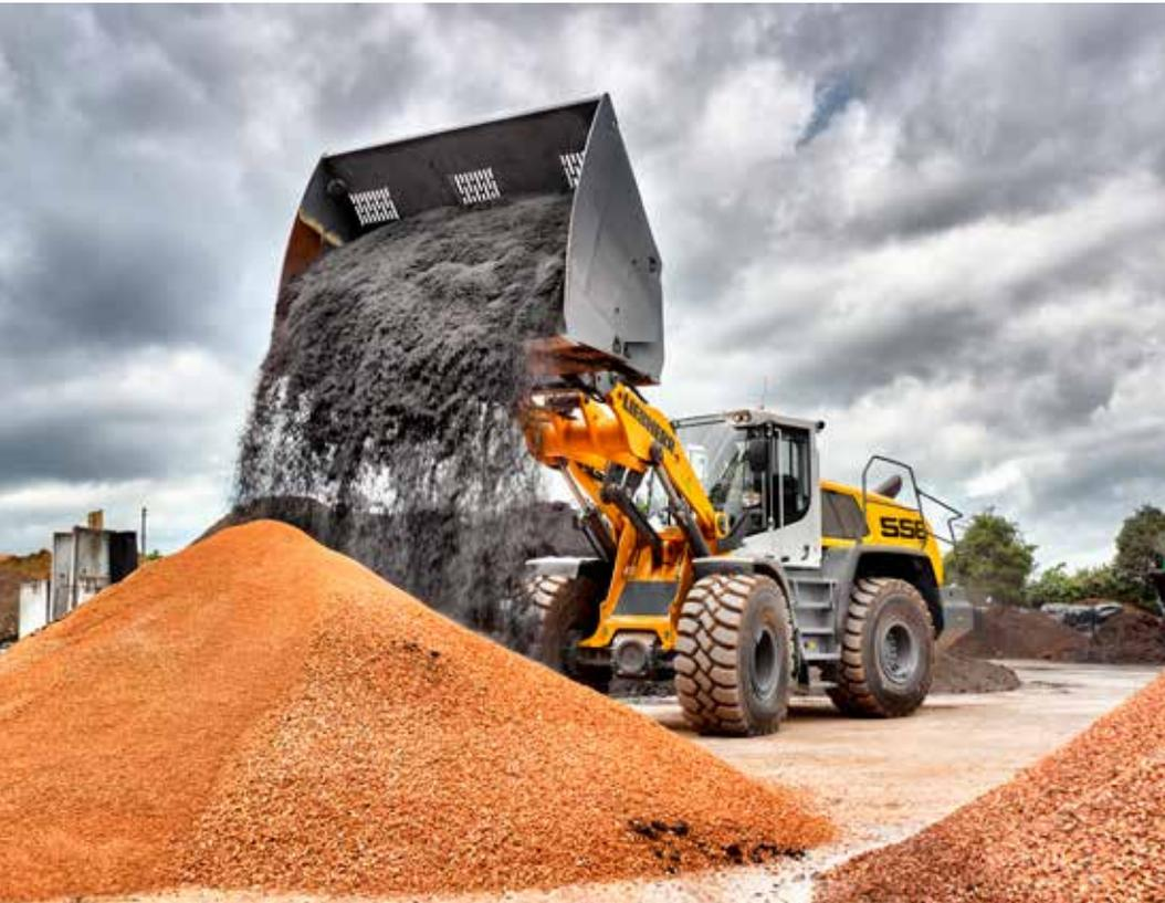
*An L 556 XPower® with industrial kinematics and high dump bucket loading soil and substrate*
